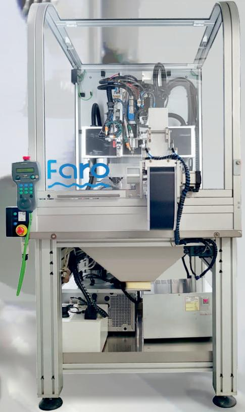
F1 is the ideal solution for productive satin finishing, engraving, diamond-cutting and final cut of pendants and of other parts to be in case bent afterwards. Available with automatic dragging device and auto alignment feature for precise machining on both sides of coils and single sheets of material.
